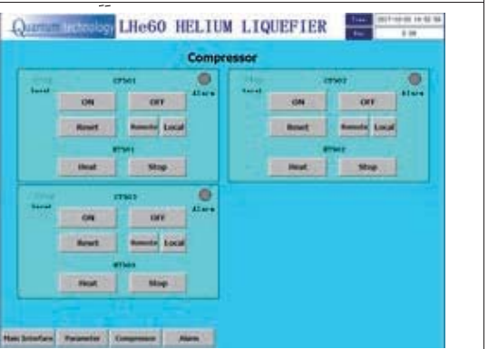
Compressor and heater control interface
