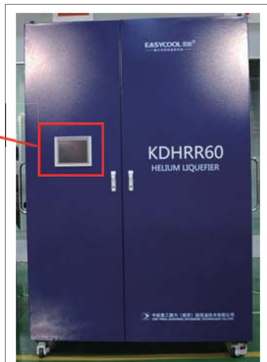
FIG.15. PLC Control Panel
