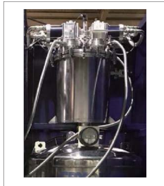
FIG.2. KDHRR60 cold box
