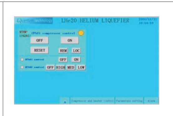
Compressor and heater control interface
