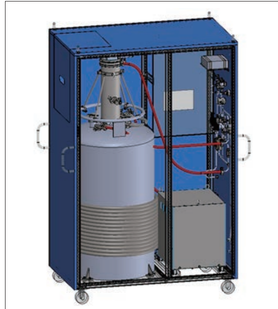
FIG.7. The whole liquefier system
